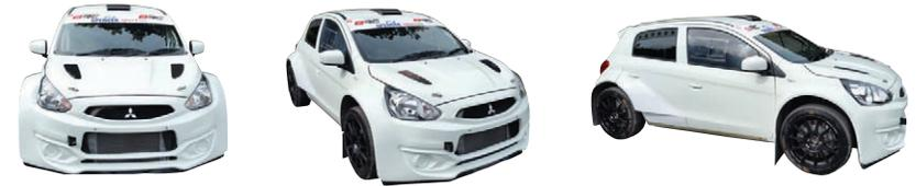
The Mitsubishi R5 is built precisely to FIA R5 Class specification. It features a 1620cc engine based on the Mitsubishi 4B11 unit from the Evolution X, connected to a five-speed Sadev transmission and four-wheel-drive system. The car is fitted with MacPherson suspension and Öhlins dampers all round, mated to specially designed subframes.
